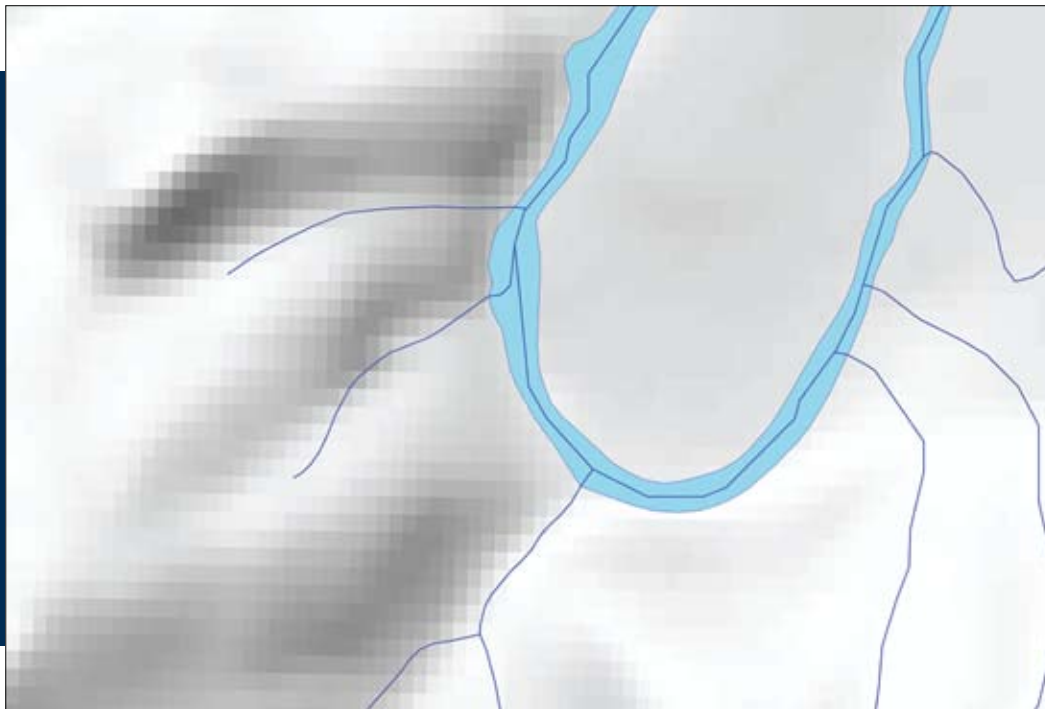
Figure 3 Hillshade and hydrography displayed at 1:24,000 scale. Note how hydrography matches terrain (hillshade) in most areas.
