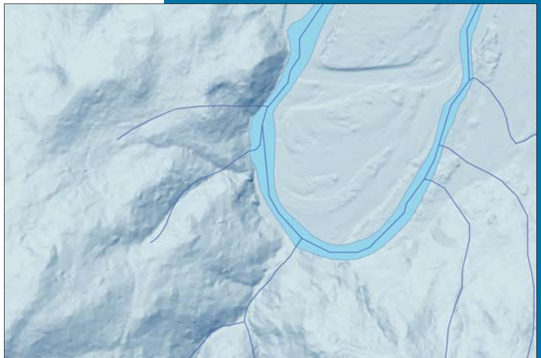
Figure 4 Enlarged area displayed at 1:2,400 shows slight discrepancies between hydrography and terrain.
