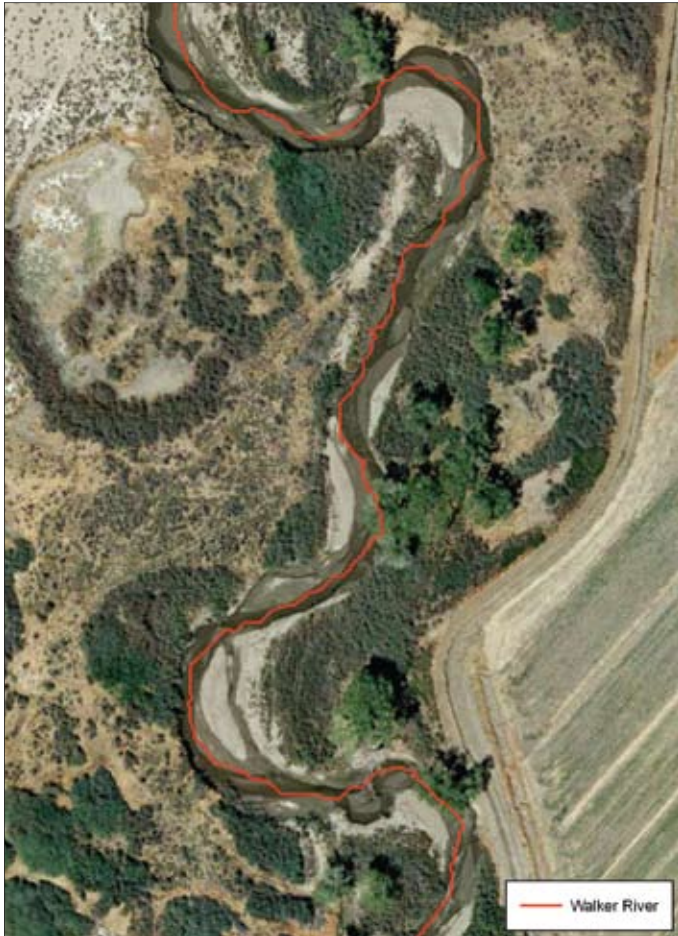
The figure on the left is a 0.3048-meter-resolution aerial photograph of the Walker River in Nevada. The image on the right is the height-above-river map using a 300-meter kernel size and classified into 50-centimeter vertical intervals. In the upper left-hand corner is a eutrophic oxbow lake that is low lying yet disconnected from the river channel. Near the bottom of the map is a shallow river channel that periodically fills with water, cutting off the point bar. An irrigation ditch is visible on the right-hand side of the image.
