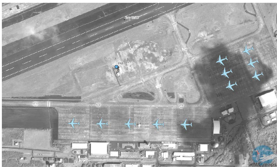
↑ Air Mobility Command's Geo Integration Office develops plans for determining the usability of an airfield for future missions. This image shows an aircraft parking plan for C-17 Globemaster IIIs on the airfield in Iwo Jima, Japan.
