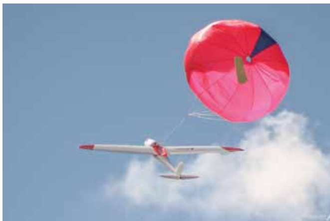
↑ The Hawkeye UAV lands by parachute, a far safer method of making an emergency landing than a belly landing.
