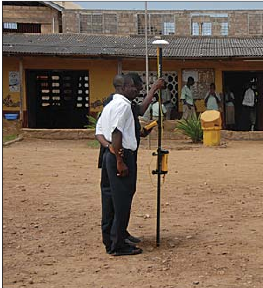
Ghanaian surveyors perform a cadastral survey of the property boundaries as described by the occupant, as well as neighbors.
