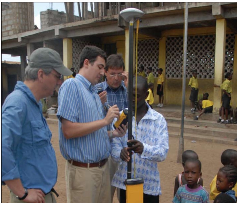
Mobile GPS-based GIS was used to survey Ms. Adamah’s school.
