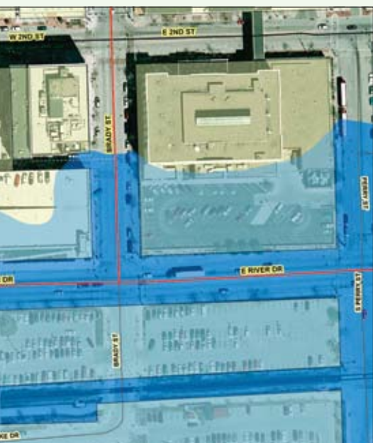
GIS flood model predicts how Mississippi River rise will impact Davenport's downtown area.
