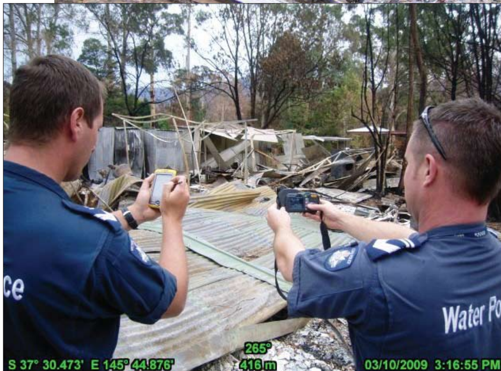
PDAs and GPS-enabled digital cameras were used to document properties searched during Operation Royals. The camera embeds the time/date stamp, coordinates, and geographic orientation into the image (see bottom of photo above).
