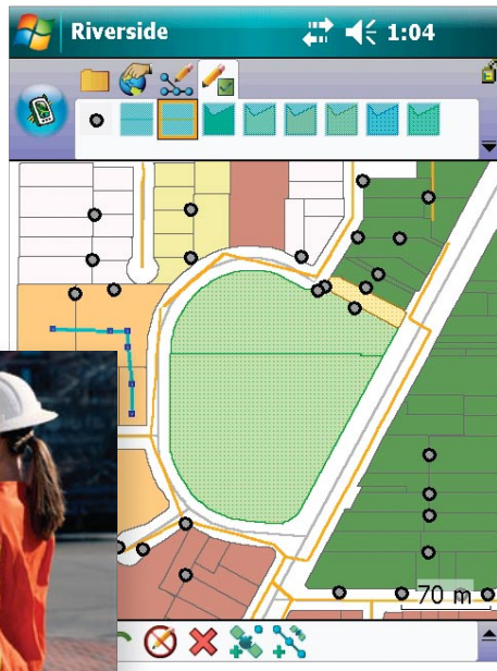
The new, dynamic QuickCapture toolbar in ArcPad 10 lets users quickly capture new features with a single tool selection.
