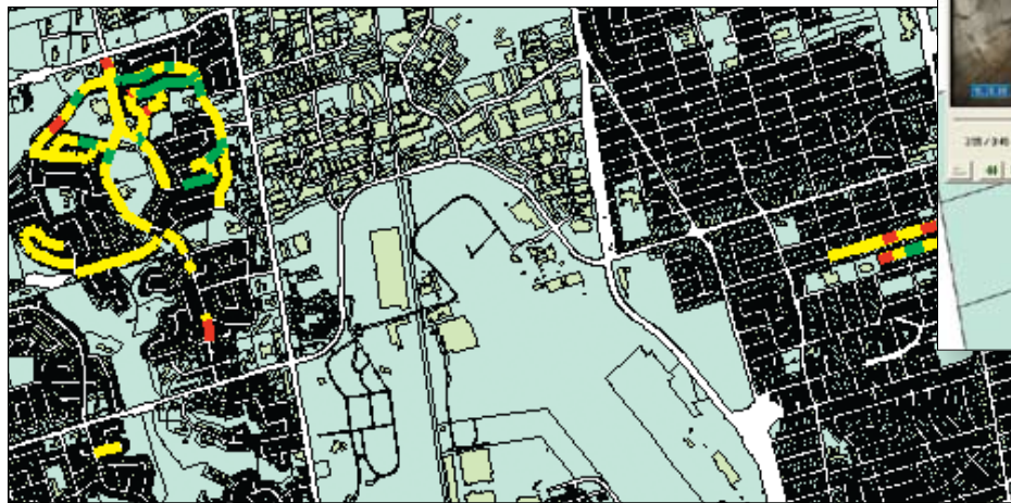
In this view of the City of Toronto, the colored layers highlight the status of the assets. For example, yellow pipes have already been inspected, green pipes require cleaning, and red pipes are in danger of a possible collapse. Above right: The inspection application's video feature lets users simply click on an asset within the GIS to pull up a video of the asset.
