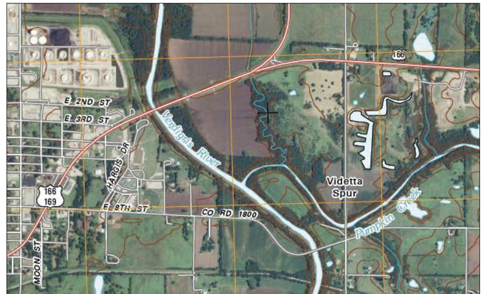
The new USTopo product includes hydrography, geographic names, elevation contours, and orthophotos.
