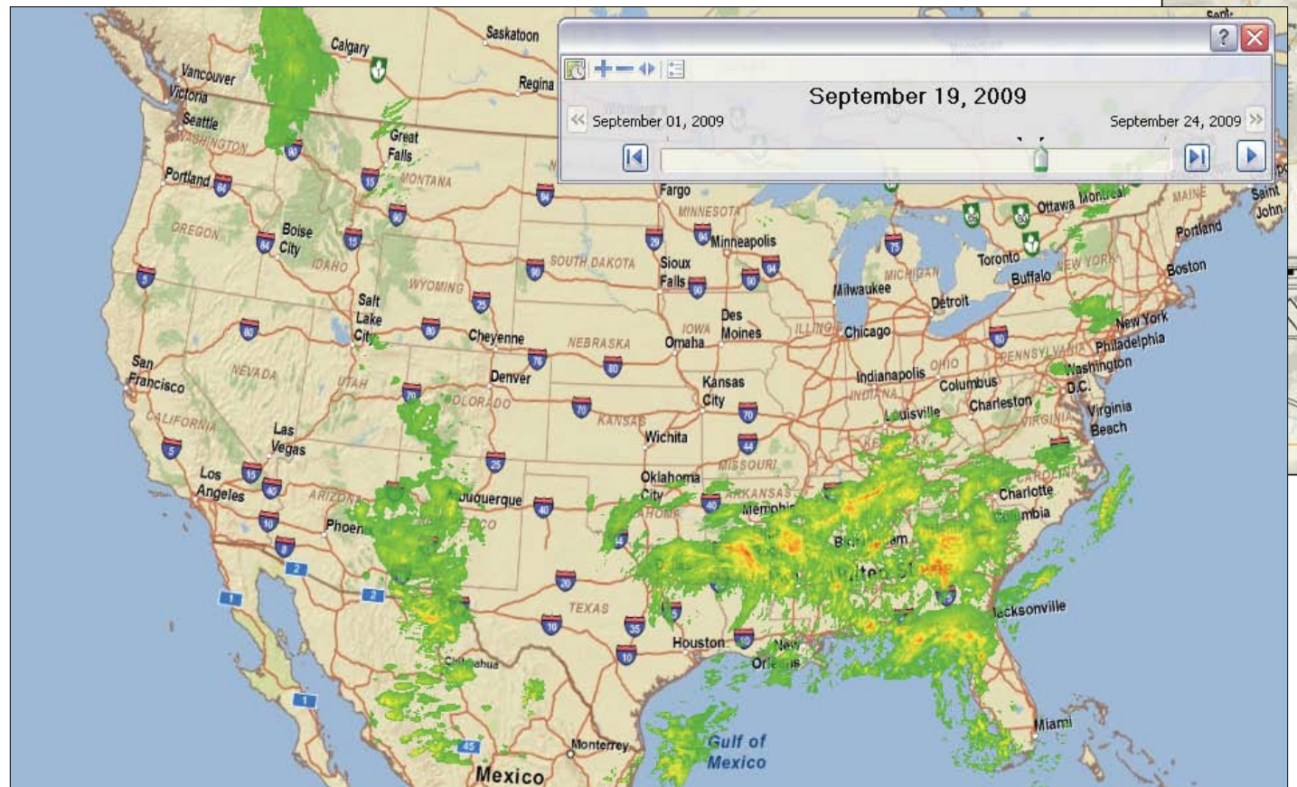
You can control visualization of temporal data in ArcGIS 9.4 using the new “time slider.”
