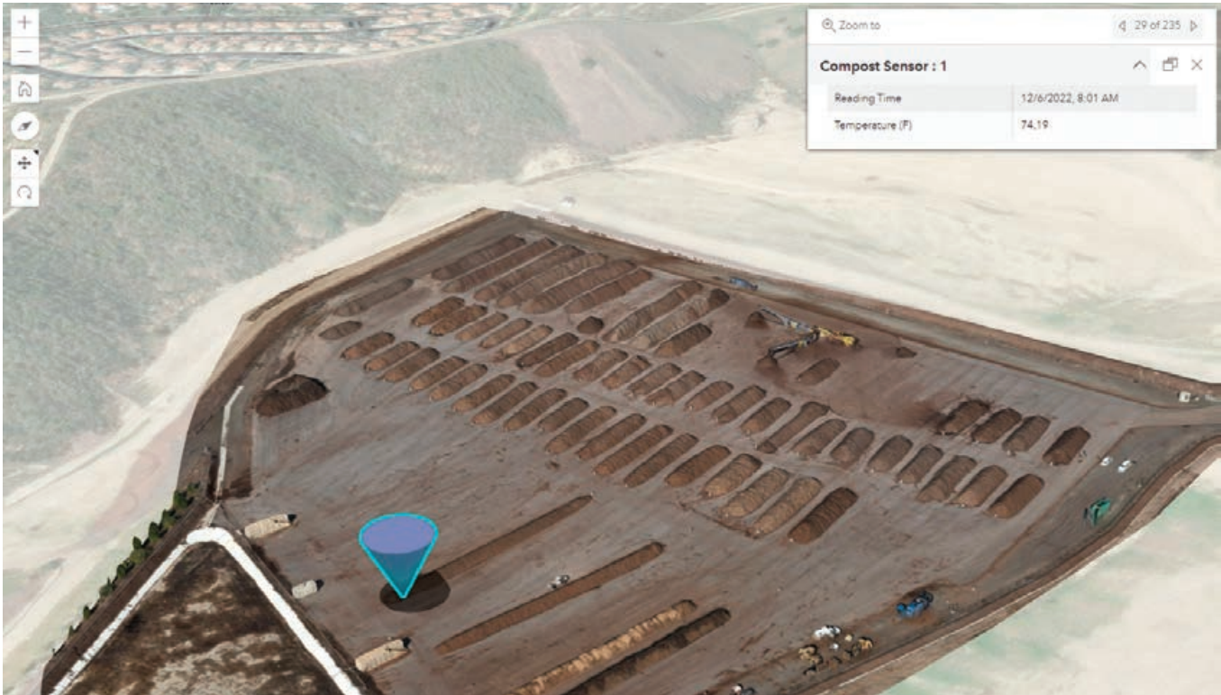
↑ A 3D web scene showing stockpile sensors lets landfill staff retrieve real-time temperature data for each stockpile by clicking on the interactive map. Using ArcGIS Velocity, staff quickly set up the sensors to feed temperature data to maps.
