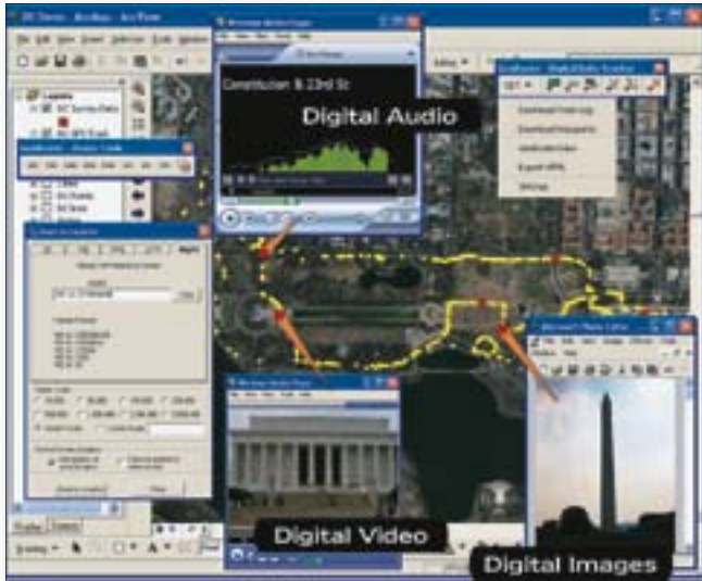
The GeoRover Digital Data Tracker extension automatically georeferences and plots data collected in the field as layers in ArcGIS. The GIS display can be converted to a Web page with one click. GeoRover software provides an interactive interface for the data to be accessed, analyzed, updated, and disseminated.
