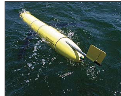
Two views of the Slocum Glider autonomous underwater vehicle.
