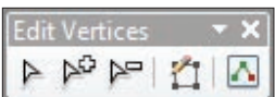
Use the Edit Vertices toolbar to move, add, or delete vertices and complete sketches.
