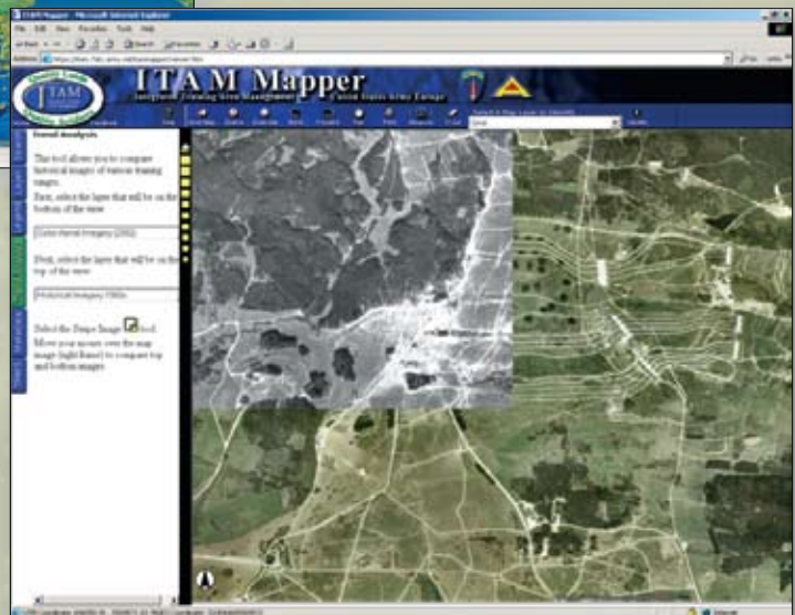
Trend analysis function allows users to dynamically “swipe” temporal data. In this example, Grafenwoehr’s Range 301 black-and-white image from 1963 is swiped over the 2002 color image.
