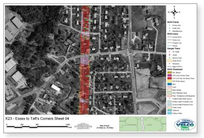
The VIP solution displays a section of transmission line with right-of-way points and lines along with dangerous trees and areas to be treated.
