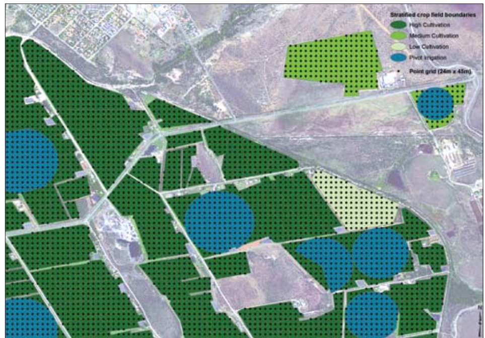
A section of the 45- by 45-meter point grid after the removal of grid points outside the crop field boundaries. Crop field boundaries stratification is also shown.
