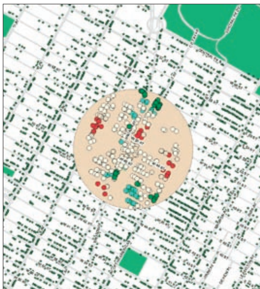
The ArcGIS modeling environment, ModelBuilder, simplifies the process of creating complex models that can be used to answer key questions. In this example, the model shown takes into account proximity to key employees and proximity to major roads and existing customers. These factors were evaluated and compared to available listings. The result is a list of potential temporary locations that meet the criteria.
