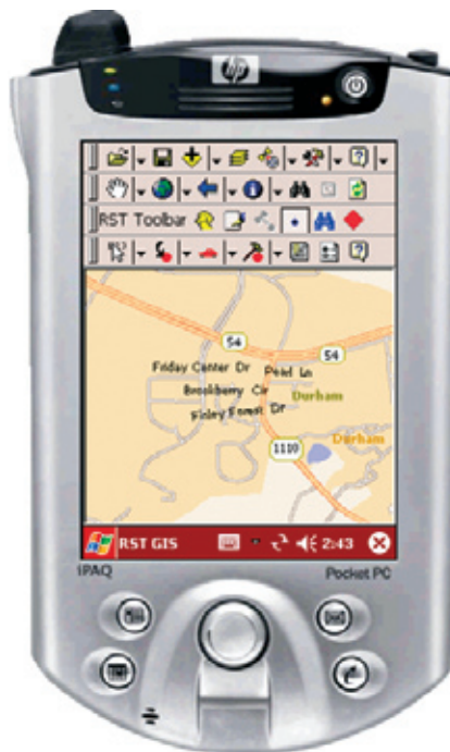
Mobile unit with ArcPad and ArcPad StreetMap installed displays a map of the survey area.
