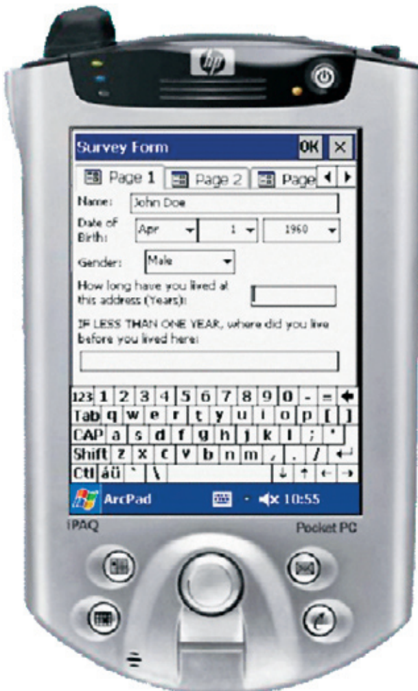
Mobile unit with ArcPad installed displays a preformatted questionnaire and allows rapid field data entry.
