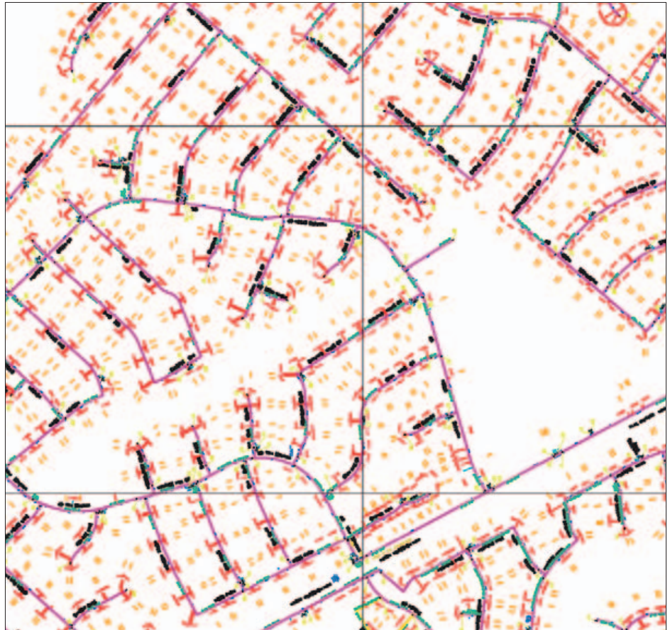
The GIS team converted hundreds of MicroStation-based water/sewer map layers, such as this one, into GIS-based, spatially accurate map files that support the asset management system.
