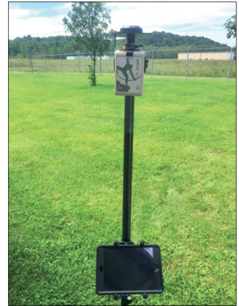
↑ Arrow 100 GNSS Receiver Mated with an iPad Mini
