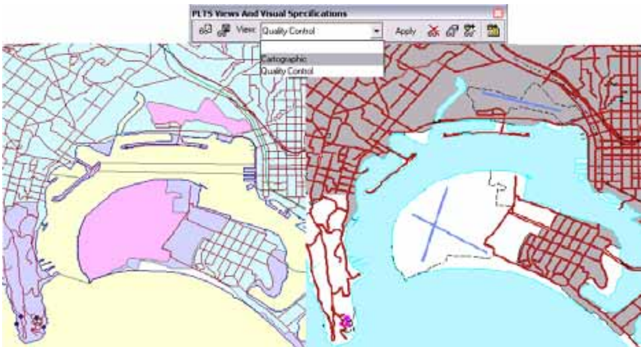
Storing PLTS views in Product Library makes it easy to apply stored layer symbology.
