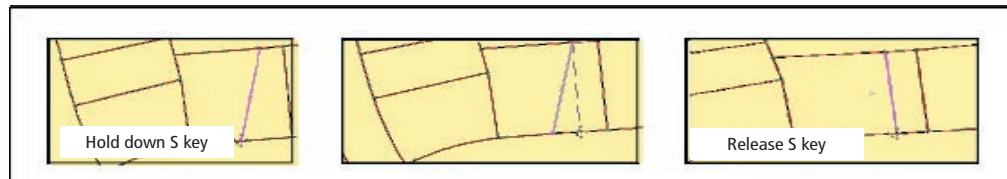
Figure 10: The Topology Edit tool allows you to move the shared boundary between two parcels without rubberbanding the connected edges.
