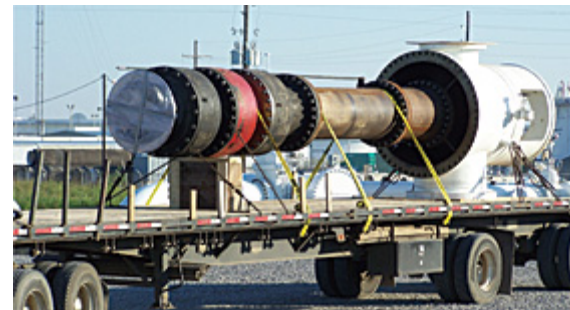
This pump at the St. James Terminal has a 27,000 barrel-per-hour capacity.
