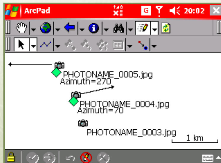
Figure 5.7 Graphics layer (arrows showing photo direction) and photo layer (camera symbols) in ArcPad.
