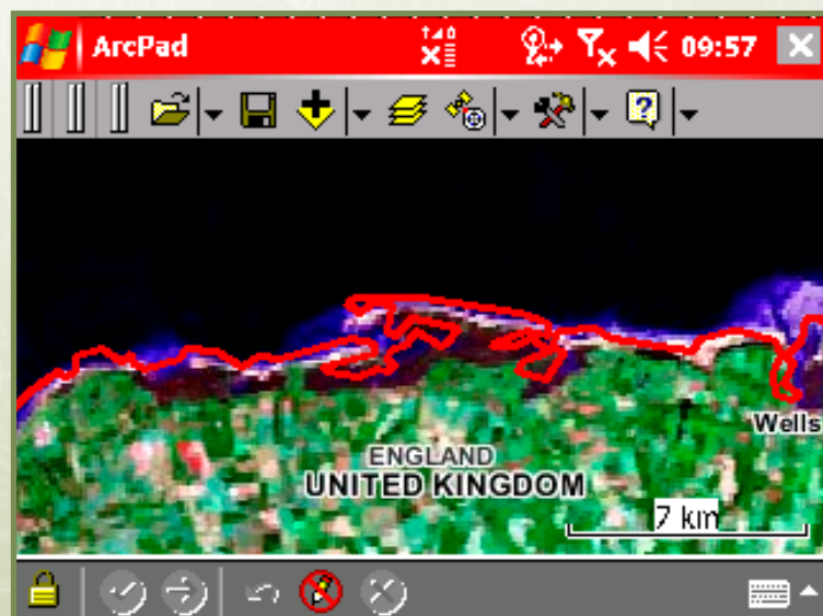
Figure 5.13 Overgeneralization of the vector coastline has led to a poor fit with the underlying image.
