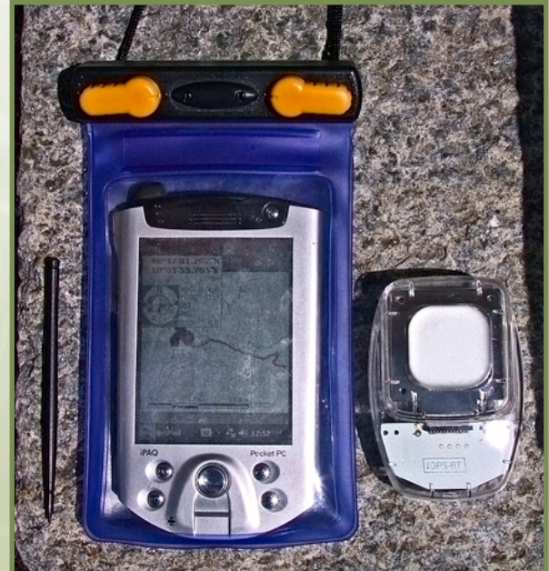
Figure 2.16 Mobile device in waterproof bag with Bluetooth GPS.
