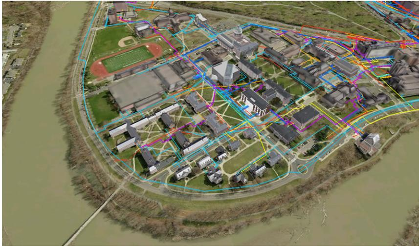
Using the ArcGIS 3D Analyst ArcGlobe software, hundreds of existing utility plans and as-built drawings were georeferenced and converted into file geodatabase feature classes in a seamless layer for each system, greatly simplifying the internal "call-before-you-dig" process. (Aerial imagery from Pictometry International)
