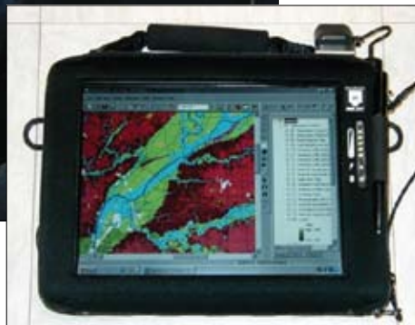
GIS loaded on a ruggedized Tablet PC allows users to view specific data in the field to determine soil characteristics and perform analysis.
