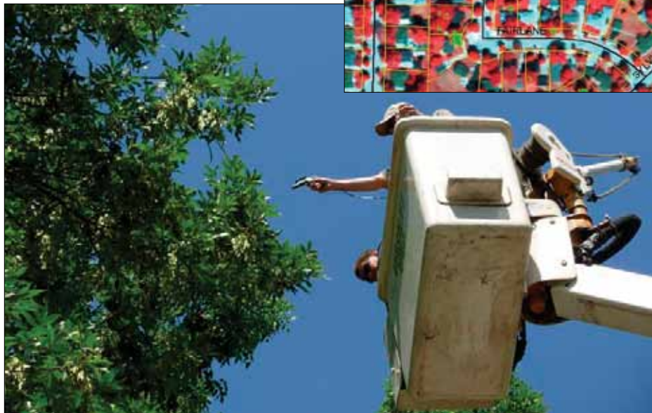
Aloft in a lift truck, city foresters use handheld spectrometers to capture canopy-level spectral signatures. This improves the accuracy of detecting ash tree species and segmenting them in 4-band multispectral imagery of the forest canopy layer.
