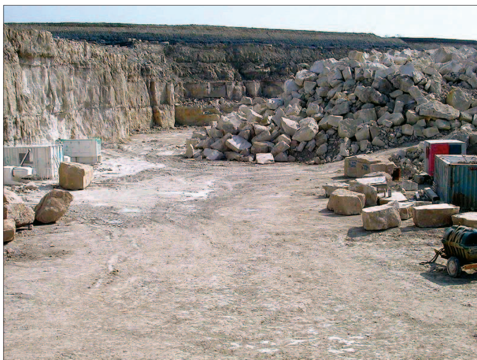
Portland stone, which is oolitic limestone, is extracted from this quarry on the Isle of Portland in the English Channel. (Photo by Mark A. Wilson, Department of Geology, the College of Wooster)
