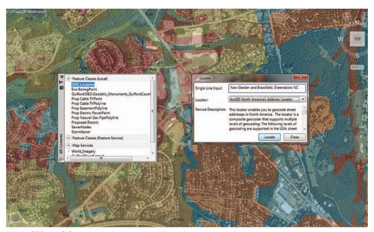
↑ Use ArcGIS for AutoCAD to access a geolocation service and locate place-names in your drawing.
