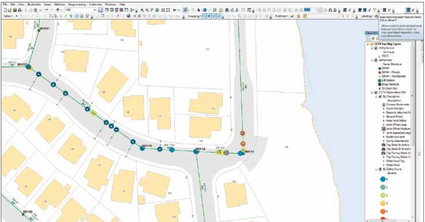
↑ By coding the severity of pipes needing repair, managers can prioritize work orders. Orange and red indicate the most severe problems. Field-workers can use the map interface to view inspection videos and other observation information.
