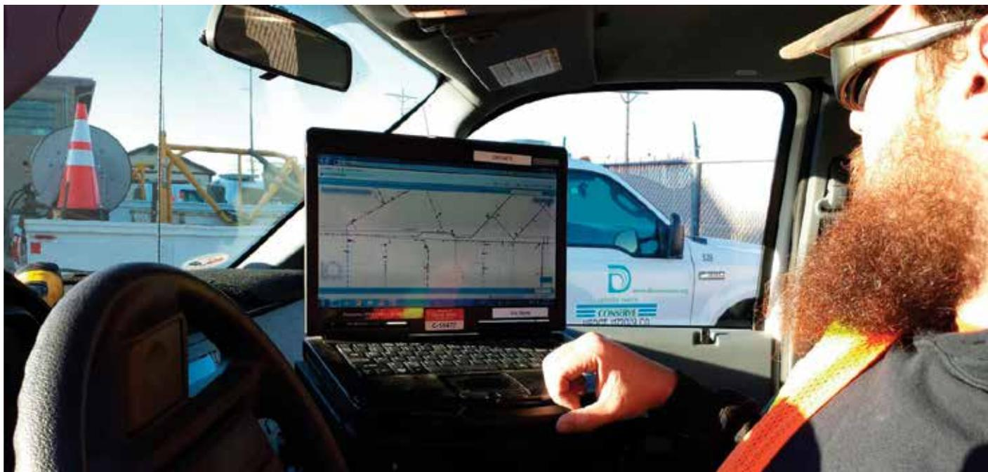
↑ A field-worker taps directly into the E-MAP GIS via a truck-mounted Toughbook. Using the GIS Pipe Network Viewer in the familiar Windows presentation, he sees the entire pipe network, including feature information, and uses GIS functionality, such as zoom and pan, at will.
