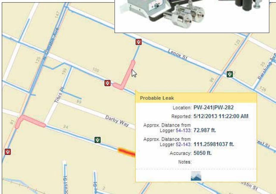
↑ Echologics acoustic technology locates leaks and displays them using an ArcGIS web application.
