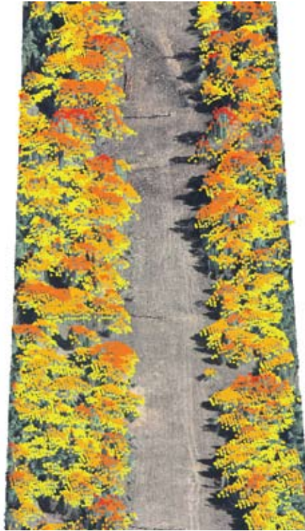
Tree height values in infrared are displayed as points created from the digital imagery. ArcGIS 3D Analyst is used to identify tree canopies that put power lines at risk.
