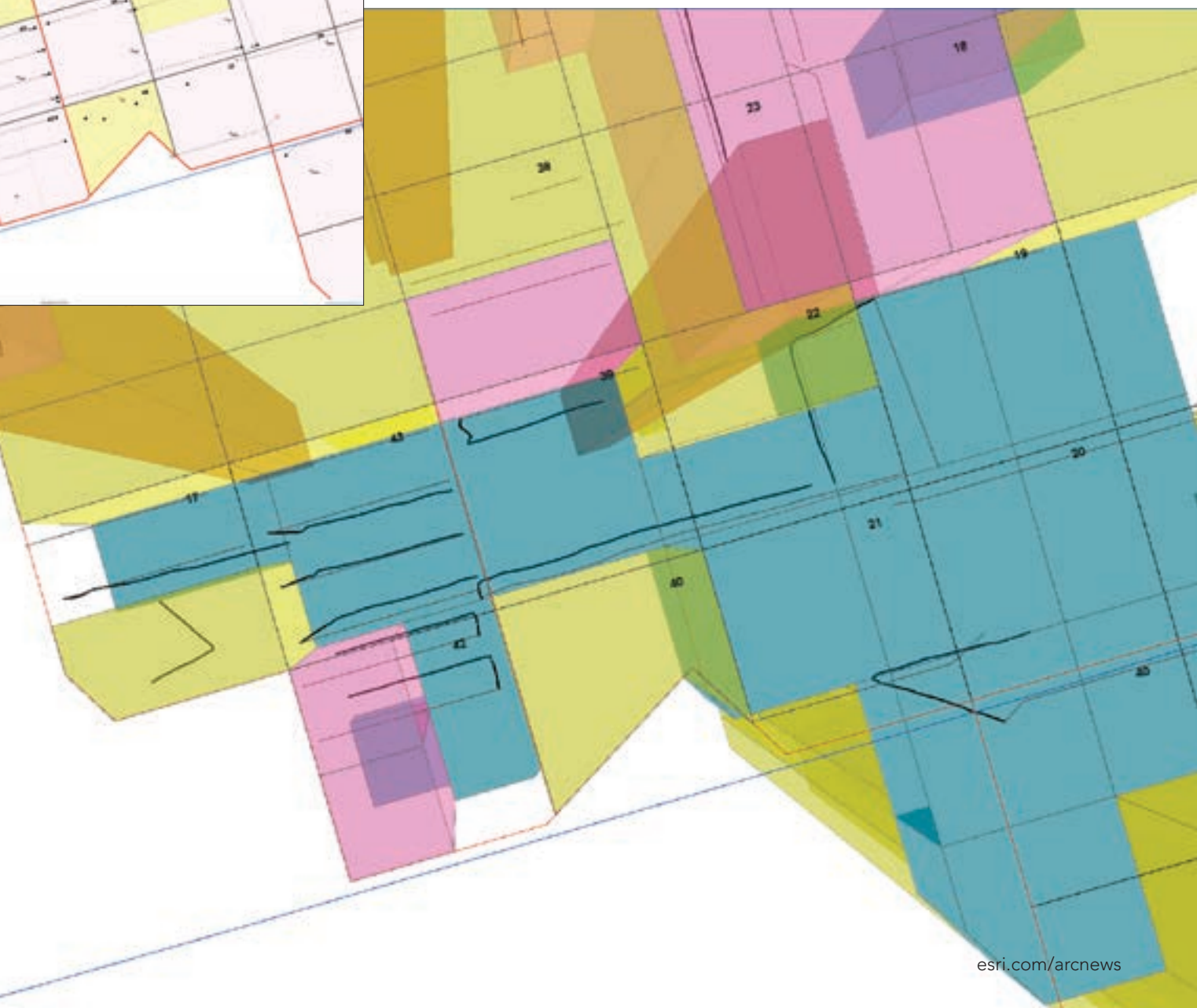
→ This map shows the wells, laterals, and leases in 3D, making it easier to see the depths of the mineral deposits and the horizontal wells (laterals) being used to extract oil and gas.
