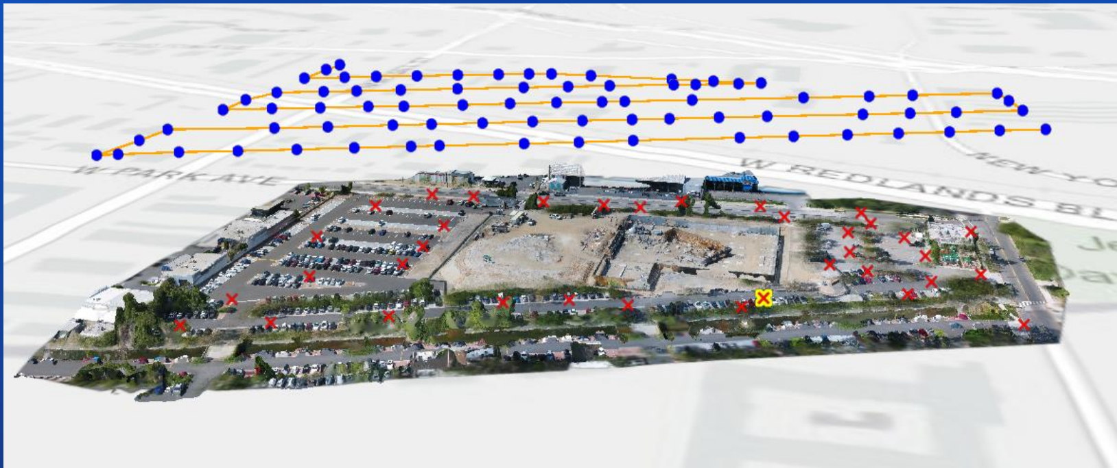
Control Points + Drone Flight Path + Orthomosaic
