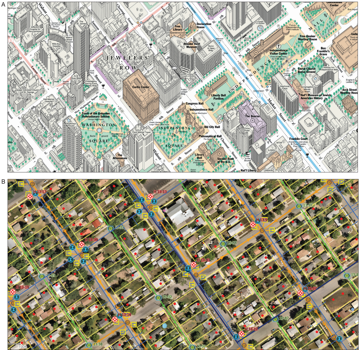
Figure 6.1. Although both of these maps show many of the same features, they are designed for different purposes, audiences, and conditions of use. As a result, the tour map (A) is pictorial and eye-catching, whereas the water utility map (B) is minimalist and utilitarian. Courtesy of Bill Marsh, Marsh Maps (A), and Jeff Sprock, City of Billings, Montana (B).
