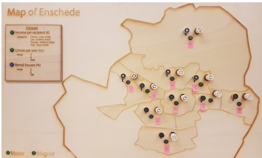
Figure 4-2. Implementation of a thematic map using the haptic kinesthetic variables of resistance and friction. The magnet is at the left and the spinning wheel is at the right of each neighborhood’s symbol group. Image courtesy of Sander Dullaert.
