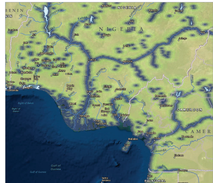
A proximity map showing distance from each cell or pixel to a reliable water source in a portion of West Africa. Water access is vital for humans as well as wildlife habitat. Streams are overlaid on the distance grid. Cells in the grid that are closest to water are darker blue. Colors change as the distance from water increases.
