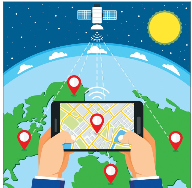
Figure 1.2. GPS consists of a receiver unit, ground control stations, and a constellation of satellites. Ground control stations track the precise location of satellites. Location is determined by measuring the time it takes radio signals to travel between a receiver unit and satellites with known locations. Image by Art Alex. Stock vector ID: 532342483, Shutterstock.
