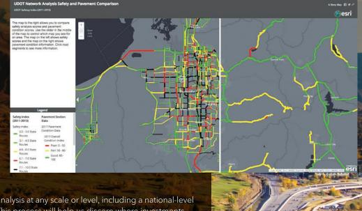
With GIS, agencies can conduct this analysis at any scale or level, including a national-level view of our transportation networks. This process will help us discern where investments would significantly improve the movement of goods and make national supply chains more efficient.
