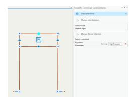
The second step is to use the Modify Associations tool to select all of the regulator station components and associate them with the regulator station assembly feature.
