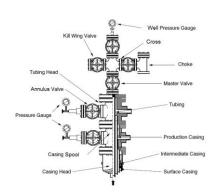
A great example of the value of supporting junction to junction connectivity is the wellhead. The wellhead diagram shown above is essentially a collection of valves and fittings. There are no pipe segments in the core construction. With the utility network's new capability to define a logical connectivity association between two point features, such as a flange and a tee, the ArcGIS system can now take a significant step forward in correctly representing this complex assembly.
