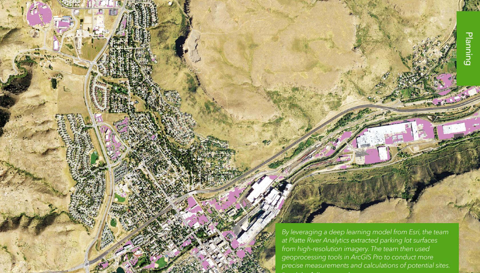
By leveraging a deep learning model from Esri, the team at Platte River Analytics extracted parking lot surfaces from high-resolution imagery. The team then used geoprocessing tools in ArcGIS Pro to conduct more precise measurements and calculations of potential sites.
