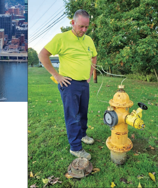
↑ An HSWA staff member uses geophone equipment to listen for noises to help identify leaks in the area.
