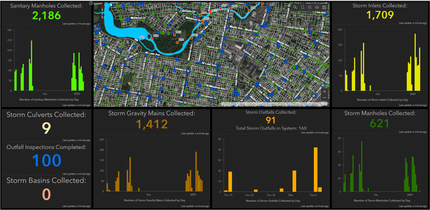
↑ As storm and sewer assets were captured with ArcGIS Field Maps and Eos Arrow Gold in the field, a dashboard created with ArcGIS Dashboards updated office personnel on what data had been collected in real time.
