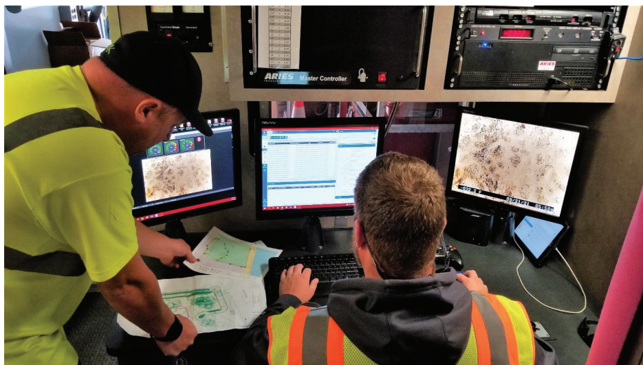
↑ Sheboygan field crews inspect underground pipes using ITpipes Mobile.
