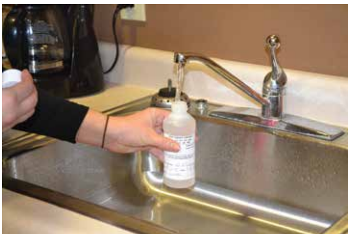
↑ Water samples are collected from the tap and tested in a lab for arsenic.
