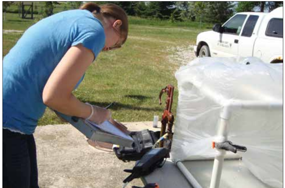
↑ GIS coordinator and environmental health specialist Sophia Walsh records field parameters for a well that is being tested for arsenic as water flows in the collection chamber.
