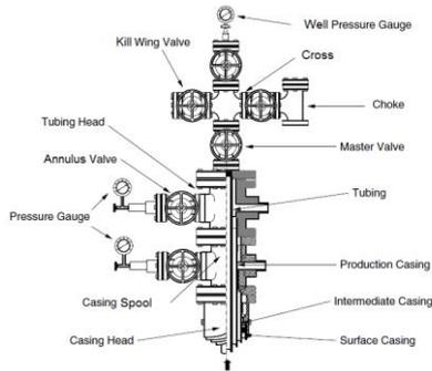
A great example of the value of supporting junction to junction connectivity is the wellhead. The wellhead diagram shown above is essentially a collection of valves and fittings. There are no pipe segments in the core construction. With the utility network's new capability to define a logical connectivity association between two point features, such as a flange and a tee, the ArcGIS system can now take a significant step forward in correctly representing this complex assembly.
