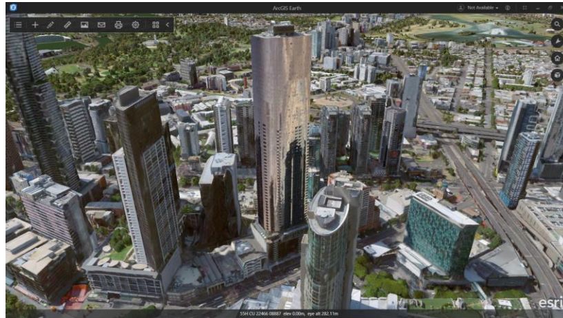
Figure 9. Software applications such as Bentley Systems' ContextCapture enable users to produce textured meshes with predictable GCI data and calculated LOS. Aerometrex used ContextCapture to create this textured mesh data for Melbourne, Australia.
