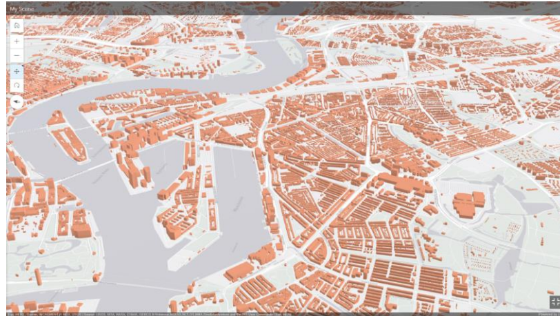
Figure 5. CityGML LOD1 buildings from Netherlands that are classified as an untextured GCI A dataset. Models are stored as I3S which intrinsically contains multiple Levels of Simplification that are not equivalent to CityGML LOD. Within the I3S, organized into nodes, the complexity rank is effectively GCI E.
