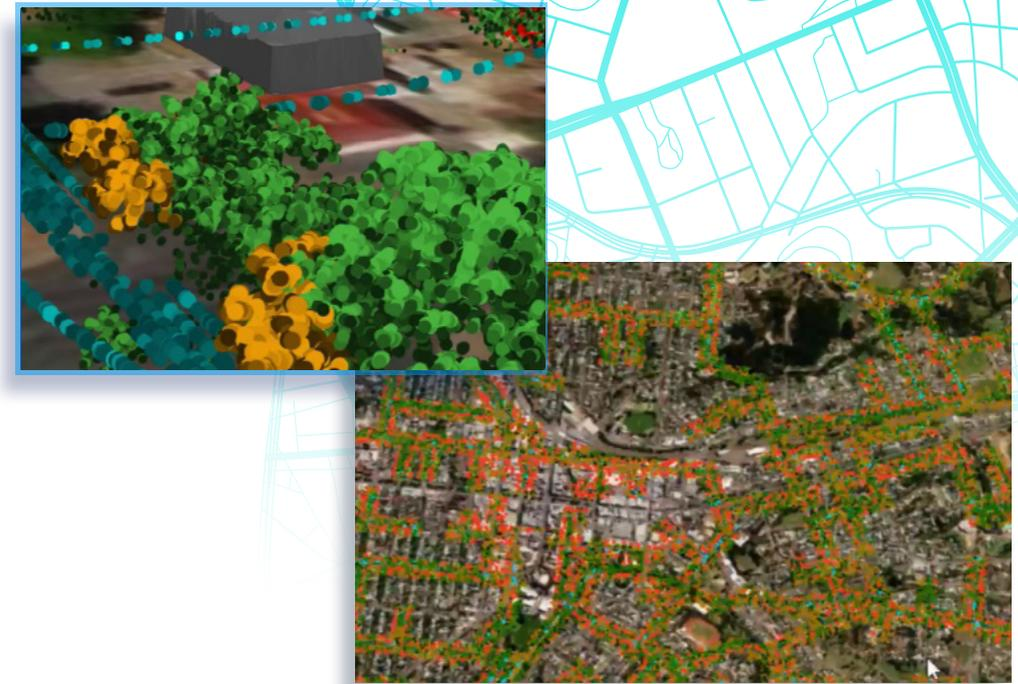
Using ArcGIS, accurate 3D models of the power lines and vegetation are created from lidar and imagery. Vegetation can be accurately modeled in relation to the power lines. Geospatial analysis tools detect if the vegetation is above, below, or intertwined with power lines. These models also are valuable for performing change detection following significant events.
