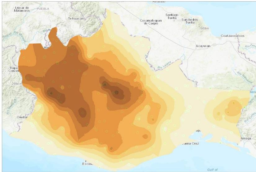
The Interpolate Points tool converted 199 elevation data points into a raster, which created a continuous surface map. The darker the color, the higher the elevation.
