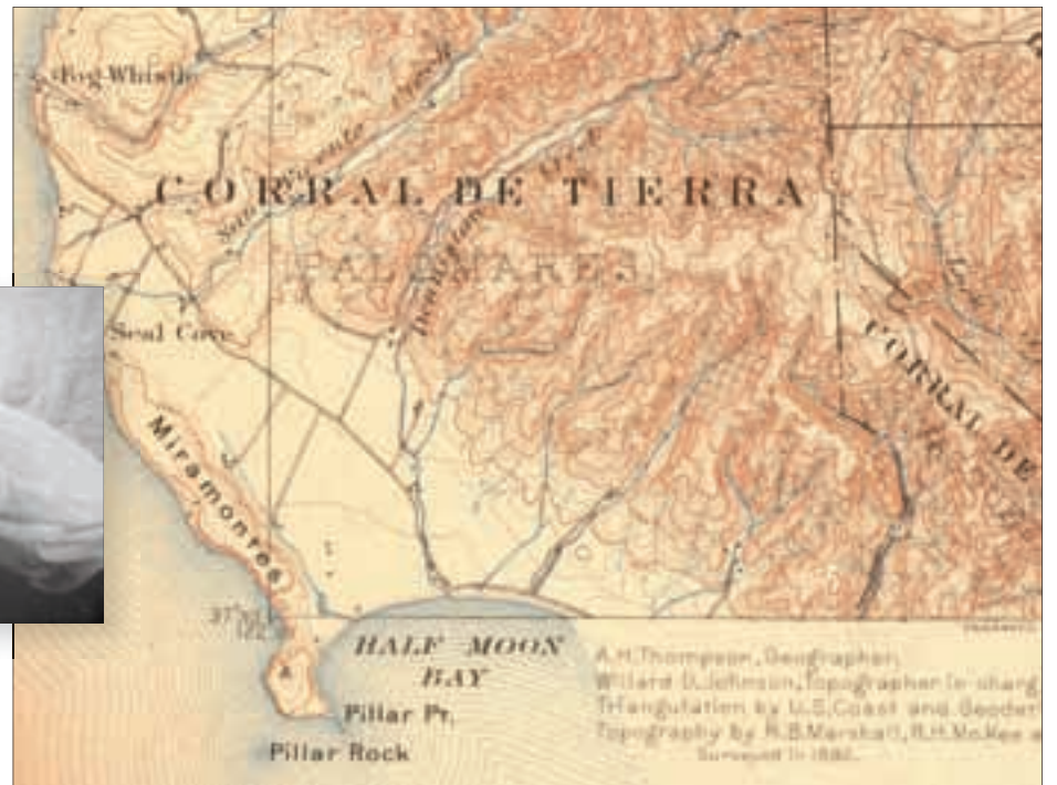
A portion of an early USGS topographic map surveyed in 1892, using contours for terrain and the water-lining method of representation for water bodies.
