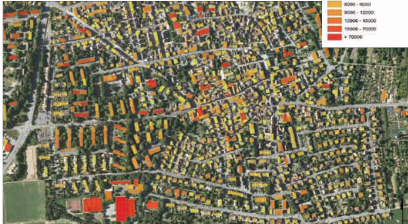
SUN-AREA researchers used ArcGIS Desktop applications to calculate the possible solar yield per building for the city of Osnabrück.
