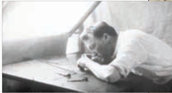
A USGS topographer engraves topographic map information onto a copper plate for map reproduction.
