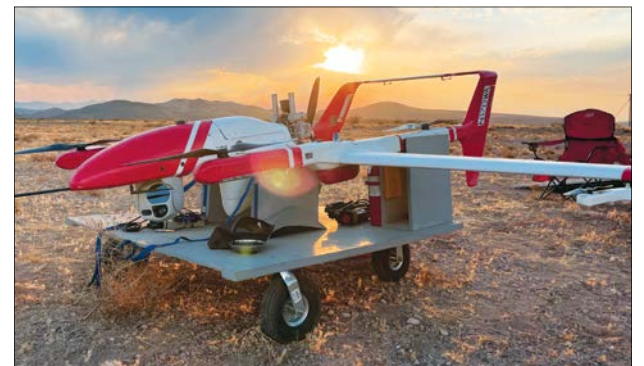
↑ Overwatch Aero's FVR-90 UAS—a fixed-wing, vertical take-off and landing, rotary drone—is equipped with a thermal, full-motion video (FMV) camera and gimbal to ensure steady imagery.
