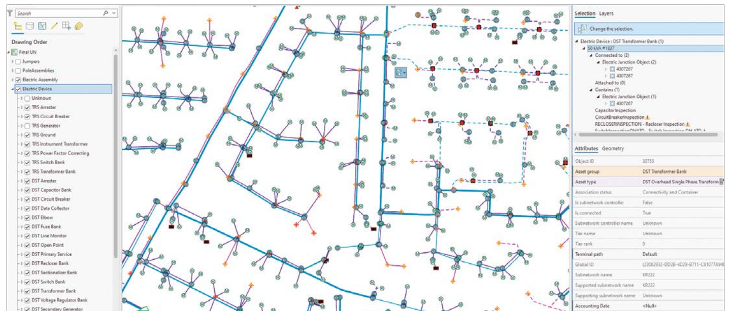
→ An ArcGIS Pro screenshot shows electric devices (distribution transformers, fuses, and switch banks) and attributes.
