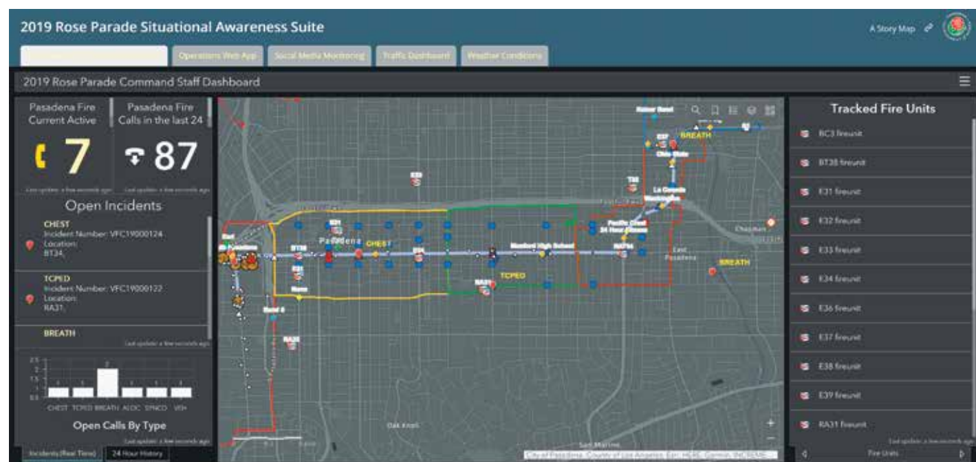
↑ The location tracks exhibited via Operations Dashboard for ArcGIS enabled dispatchers to identify the unit closest to an incident and/or pinpoint the unit that would be able to get to an incident the quickest, taking barricades and traffic jams into consideration.
